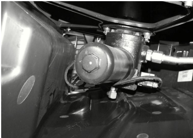
Canister style cast-iron cover for 6692337 .
