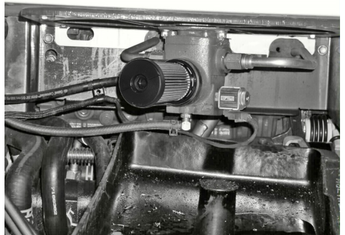
Canister style filter 6692337 with cover removed.
